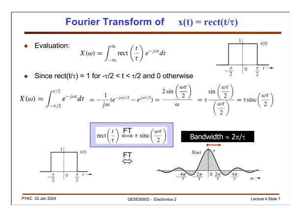
The reason that sinc-function is important is because the **Fourier Transform of a rectangular window rect(t/\tau)** is a sinc-function.
